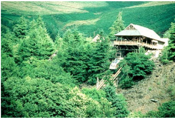
The funicular railway that brings visitors from reception to the main site, operated by gravity and water
