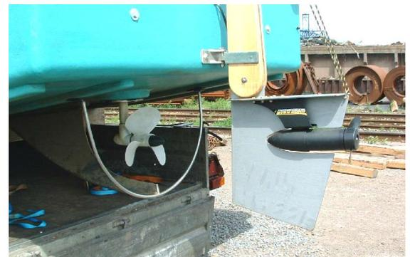
More pictures of the Escargot, showing the interior with sitting headroom, the twin pedal-drive units and the propeller they are coupled to, and also the electric outboard drive incorporated into the rudder.
