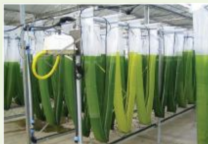
Flue gases from the Niederaussem power station in Germany are fed into an algae production plant to convert the CO 2 from the flue gas into algae biomass. [Source of picture: RWE Power].
