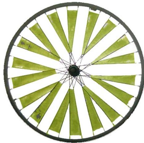
**Fig. 1** Bicycle wheel converted into a *convergent* turbine.
