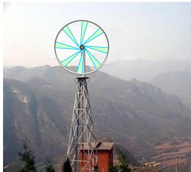
**Fig. 4** Bicycle wheel turbine mounted on a typical American mill structure. With 2 m of radius, this would receive 8 KWatt of wind power at 10 m/s wind speed.
