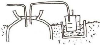
i. Connect one of the pipes in the cylinder lid with the gas barrels with a clear hose.
