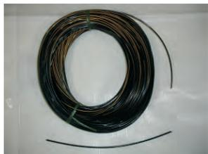
**i) Micro-tube:** Straight or curled LLDPE tube with an inner diameter ranging from 1 to 1.2 mm. The discharge from the micro-tube is directly proportional to the operating pressure and inversely proportional to its length. The operating pressure that is required can be as low as 1-5 meters.
