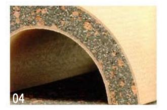
Steam heats the fibers and the soft raw material is ground into a refiner. Finally, an adhesive is added to the material, and hot-pressed to create the desired density of the fiberboard.
