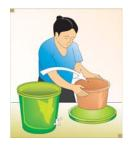
Step 3: Clean the receptacle tank and spigot with soapy water. Allow it to air dry.
