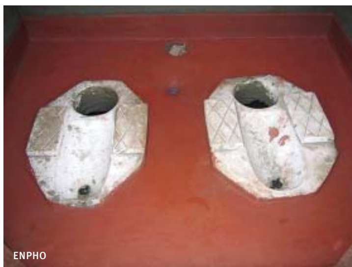
Photo 3.5: Pan for Dry EcoSan toilet
