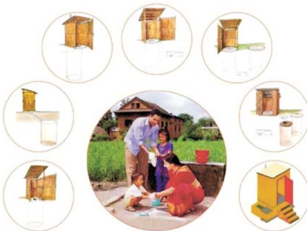
Figure 2.1: Various types of latrines: Pit latrine, VIP latrine, offset pit latrine, EcoSan toilet
