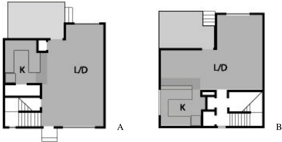
Figure 5-15. Unit plans (after Preston & Associates, 1994). Figure shows the spatial distribution of the ground floor for A) typical unit, B) custom unit.
